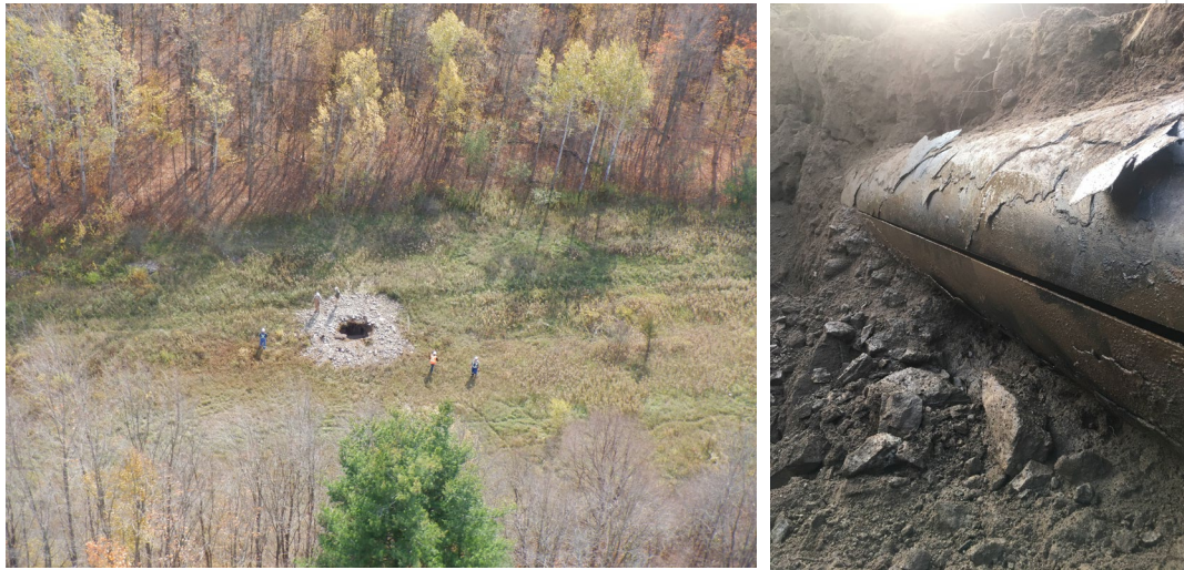
Figure 1: HydroTest failure location and ruptured pipe
