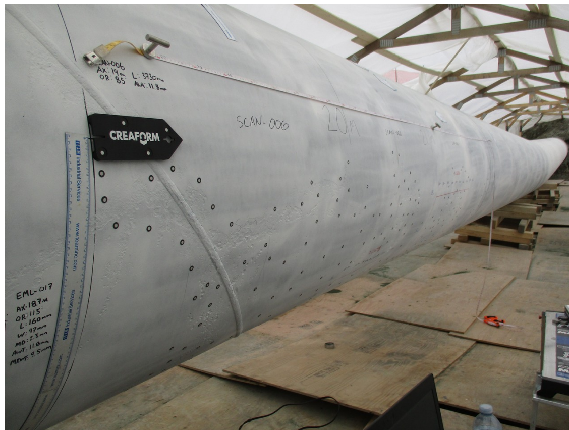
Figure 10: Field laser Scanning Corrosion feature
